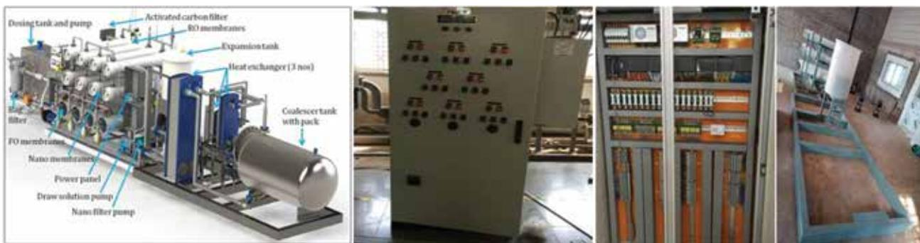
**Figure. 4. Forward Osmosis (FO) desalination system to provide potable water in Narippaiyur test bed facility**
