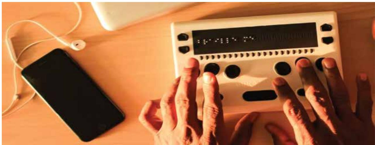
**Fig : Read-write electronic braille device (BrailleMe) at CoE, SINE- IIT Bombay**
