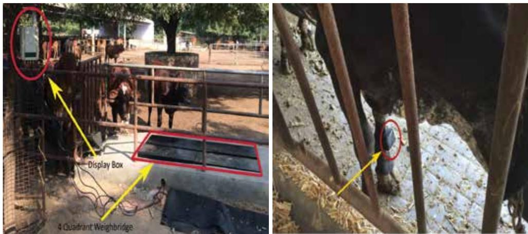
**Weighing machine installed in the campus A cow with a Pedometer on its rear left leg**
