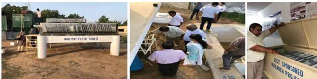
**Fig. 6. 10 KLD capacity sensitive photo catalytic filters for visible light catalysis and carbon nano-mat fiber filter developed by MNIT Jaipur and MBM College of Engg, Jodhpur for treatment of the effluent of Common Effluent Treatment Plant, in Jodhpur**
